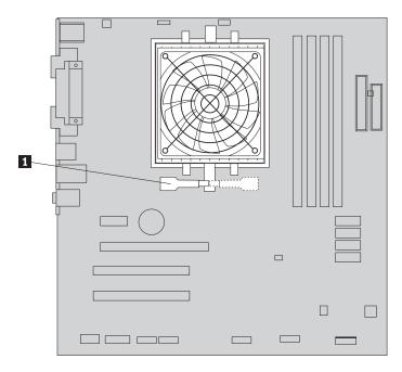
Figure 17. Replacing the heat sink and fan assembly
